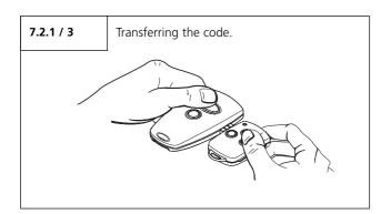
• Whilst keeping the button on the master transmitter depressed, press the desired button on the other hand transmitter. The LED flashes.
